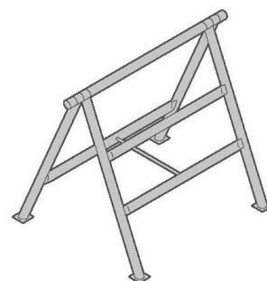
Figure 2 'A-frame' trestle scaffold
